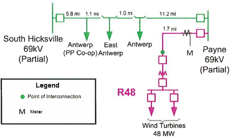
The Point of Interconnection is at the first structure outside of the Interconnection Customer's collector substation with the Interconnection Customer owning the conductors out of the substation and AEP owning the first structure.
