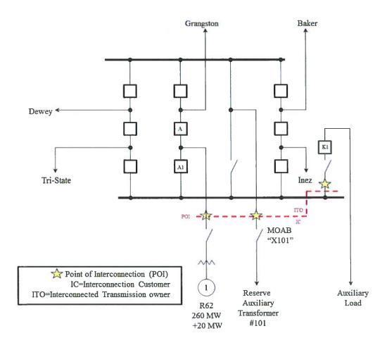
The Point of Interconnection is at the Interconnected Transmission Owner 138 kV structure in the Interconnected Transmission Owner's Big Sandy Substation with Interconnection Customer owning the 138 kV switch and other infrastructure leading to the Customer Facility.
