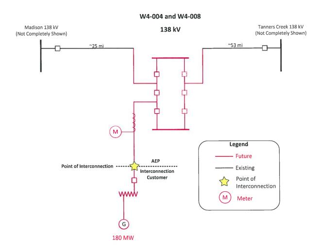
The Point of Interconnection is at the first structure outside of AEP's 138 kV switching station with AEP owning the conductors to the first structure and Interconnection Customer owning the structure and remaining facilities back to the generation collector station.
