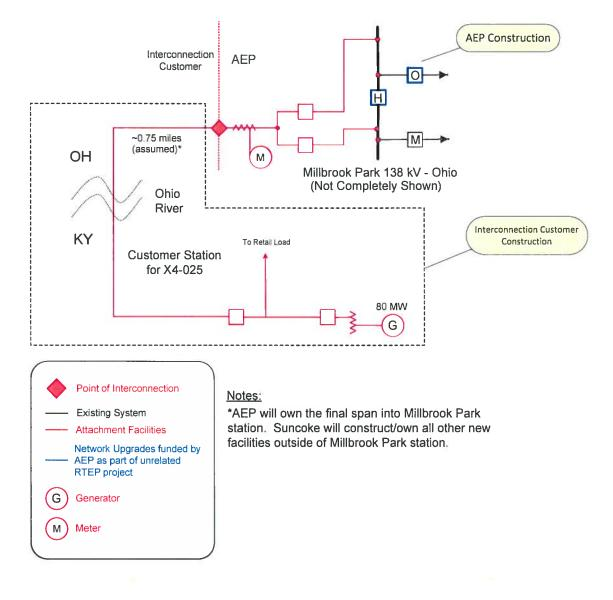
The Point of Interconnection is at the first structure outside of Millbrook Park station with AEP owning the first span of conductors from Millbrook Park to the Interconnection Customer's first structure and Interconnection Customer owning the structure and remaining facilities back to the collector station.
