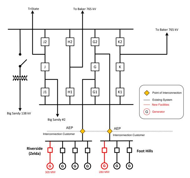
The Point of Interconnection is at the Interconnected Transmission Owner's dead end structure in Baker 345 kV substation. Interconnection Customer owns the conductors connecting to Kentucky Power Company's dead end structure and the other facilities connecting to the generation.
