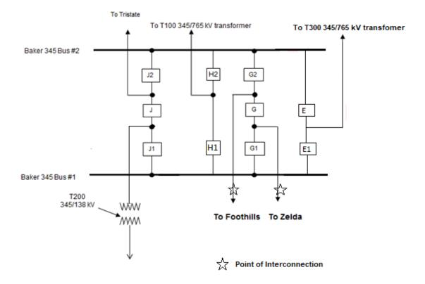
The Point of Interconnection is at the Interconnected Transmission Owner's dead end structure in Baker 345 kV substation. Interconnection Customer owns the conductors connecting to Kentucky Power Company's dead end structure and the other facilities connecting to the generation.
