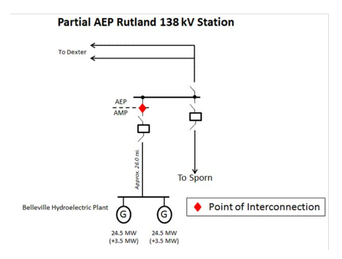
The Point of Interconnection is at AEP's Rutland station on the 138 kV bus with AEP owning the 138 kV bus and AMP owning the conductors and all facilities back to the Belleville Hydroelectric Plant.
