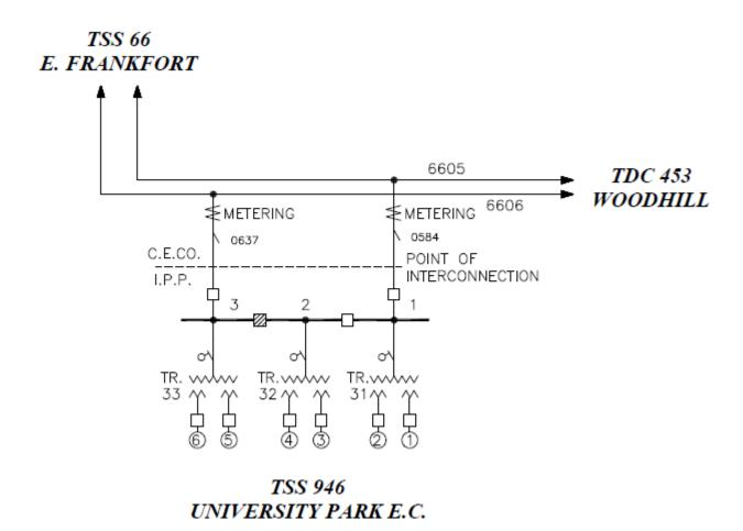
Points of Interconnection: Customer Side of ComEd 138kV Disconnect Switches
