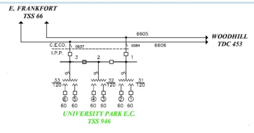
Points of Interconnection: Customer Side of ComEd 138kV Disconnect Switches
