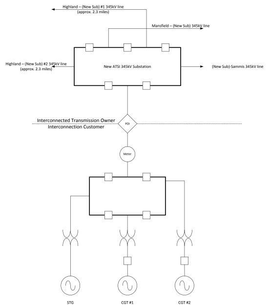
Note regarding Point of Interconnection (POI): The physical POI will be located within the interconnection substation. The Interconnection Customer-owned dead-end insulators between Interconnection Customer-provided generator attachment wire and the Interconnection Transmission Owner dead-end structure will be defined as the POI.
