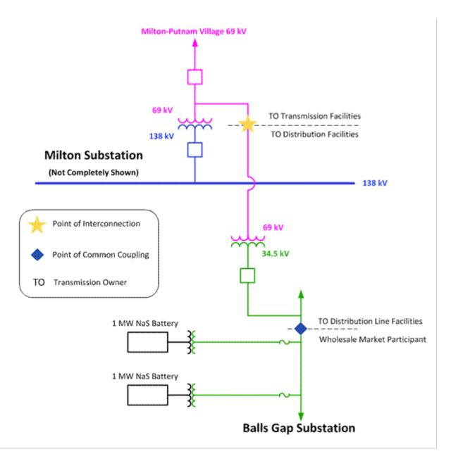
The Point of Interconnection with the transmission system is at Transmission Owner's Milton 69 kV Station between the Transmission Owner's 69 kV MOAB "W" and circuit breaker "F". The point of common coupling (PCC) with the local distribution system will remain at Transmission Owner's distribution primary pole 38820153D30115.
