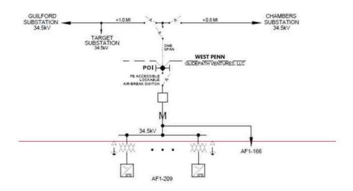
→ POI (POINT OF INTERCONNECTION) LOCATED AT INTERCONNECTION CUSTOMER'S DEAD-END STRUCTURE WHERE WEST PENN POWER'S OWNED 34 5kV TRANSMISSION LINE TERMINATES
