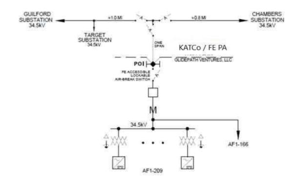
POI (POINT OF INTERCONNECTION) LOCATED AT INTERCONNECTION CUSTOMER'S DEAD-END STRUCTURE WHERE KATCO / FE PA OWNED 34 5W TRANSMISSION LINE TERMINATES
