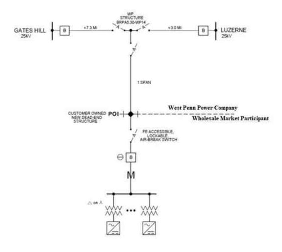
├──── POI (POINT OF INTERCONNECTION) THE POINT OF INTERCONNECTION IS LOCATED AT THE CUSTOMER OWNED DEAD-END STRUCTURE WHERE WEST PENN POWER (WP) LINE TERMINATES
