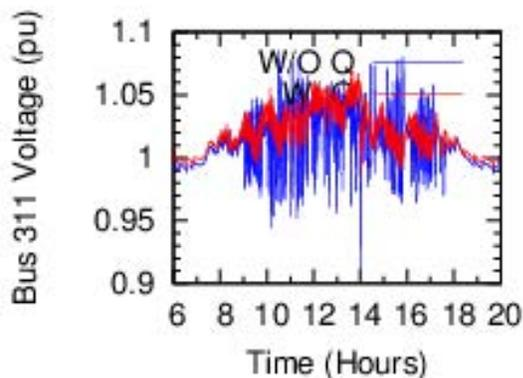
SDG&E also modeled the effectiveness of using inverter based technology plus energy storage. The results shown below indicate that using inverter based technology plus energy storage is even more effective at mitigating voltage swings than just using inverter based technology alone.
