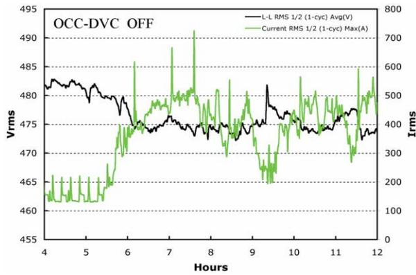
The graph below shows the transformer secondary voltage after a 240kVA inverter based device with reactive power control was installed and operated. Clearly the inverter based device significantly improves the line voltage.
